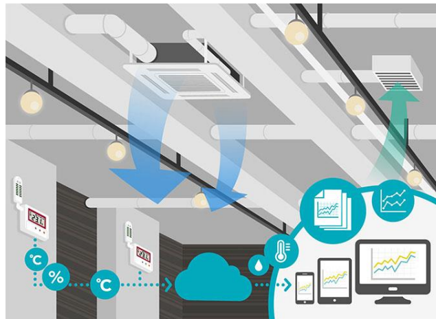
Figure 3: Supply Air and Return Air Vents for HVAC
