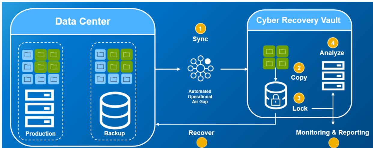
The PowerProtect Cyber Recovery solution protects the most critical data in a vault environment. The vault is ideally physically isolated – a locked cage or room – and is always logically isolated via an operational air gap. Vault components are never accessible from production, and access to the vault target – when the air gap is unlocked – is extremely limited. This is a key to the maturity of our solution (and can be covered in a separate, more technical
