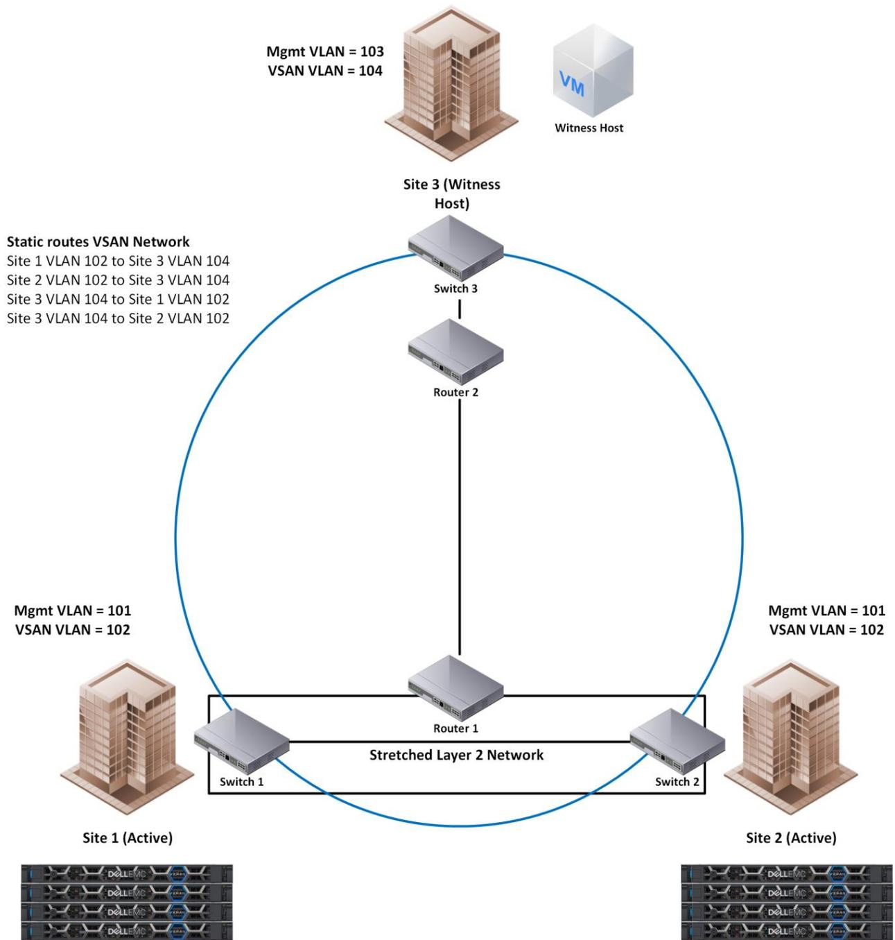
**Figure 3 - VxRail Supported Network Topology**
