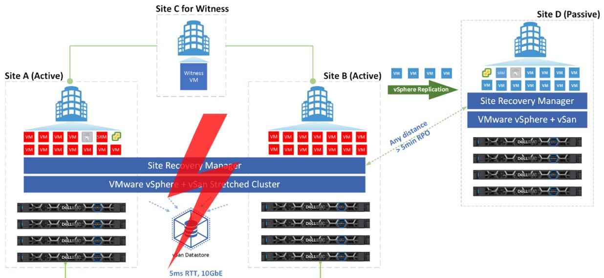
Figure 11 – All of the VxRail appliances faulted at site A and site B
