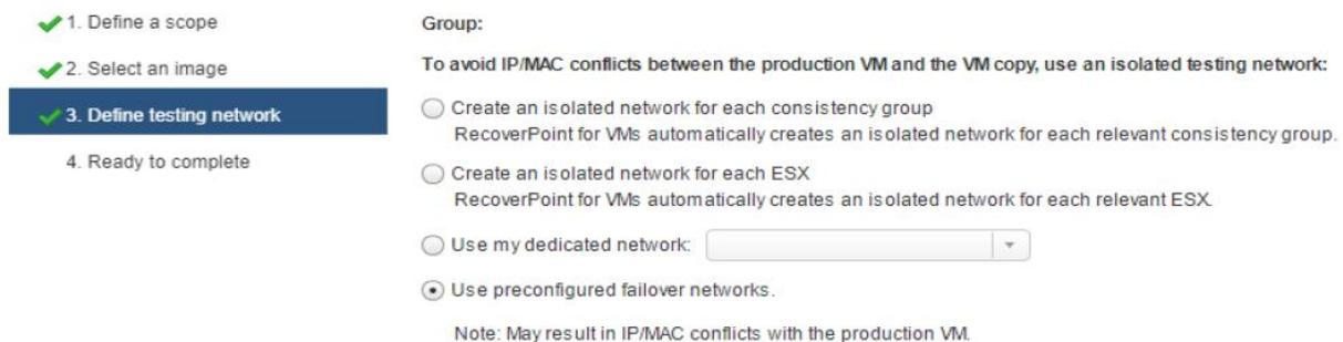
Figure 17 - Define testing network in test a copy wizard.
