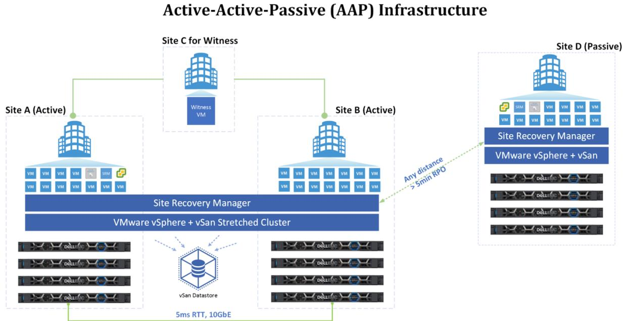
Figure 9 - Architecture Diagram of VMware vSAN Stretched Cluster with SRM
