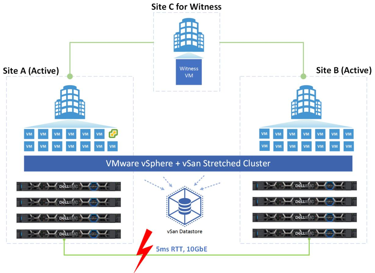
Figure 6 - The vSAN network is disconnected between site A and B
