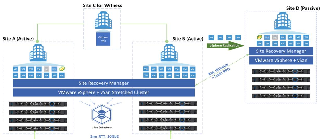
Figure 10 – The virtual machines are replicated to site D from the protected site (A + B)
