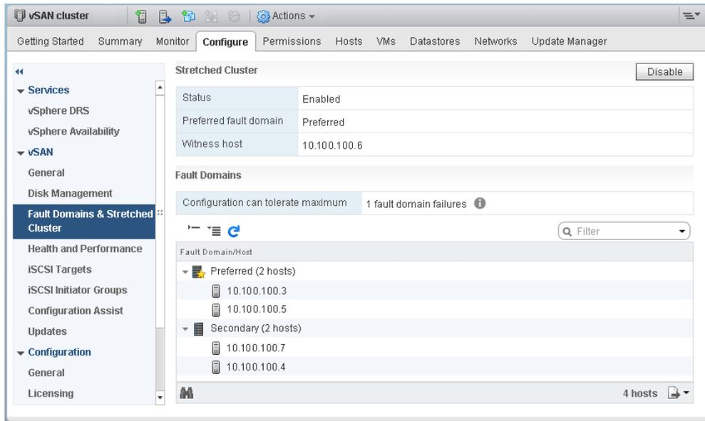
**Figure 1 - Configuration of Fault Domains & Stretched Cluster**
