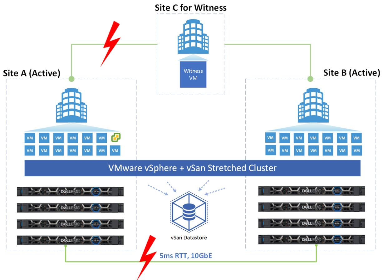
**Figure 7 - The vSAN network is disconnected between site A and B, and the witness network is disconnected between site A and C.**
