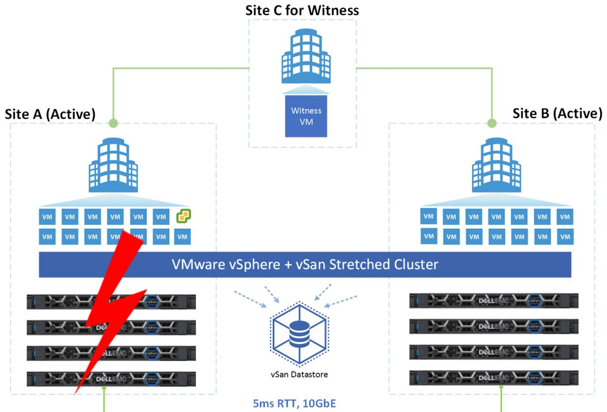
Figure 5 - All of the VxRail appliances faulted at Site A
