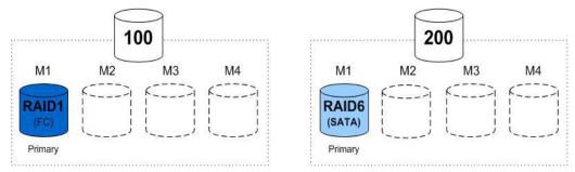
2. The configuration lock is placed on an array to perform the swap. Also, a DRV device is chosen and the associated RAID group is detached and associated with one of the devices being swapped.
