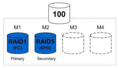
After synchronization, the lock is acquired once again and the device configuration is updated to swap primary and secondary roles of the mirror positions. Thus, the original RAID 1 mirror is demoted to secondary while new RAID 5 mirror is promoted to primary mirror.
