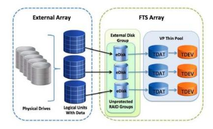
The maximum external capacity is determined by the VMAX cache. The maximum number of LUNs per external storage port is 8,000 and 14,000 eDisks per DX director port with a higher limit of 128,000 eDisks per array.
