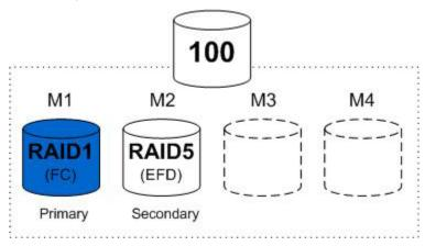
Once done, the secondary RAID group is completely invalidated to be synchronized from primary mirror and configuration lock is released.
