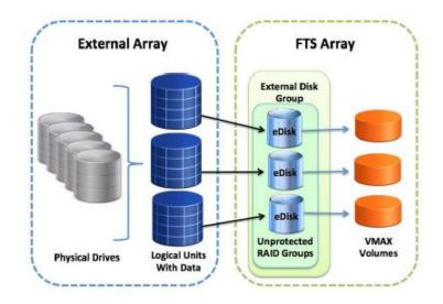
In virtual provisioning encapsulation, the eDisk is created and added to an external disk group with a virtualized RG. Thin data devices (TDATs) are then created and added to a specified external thin pool. Thin devices will be fully allocated and a one-to-one thin extent to TDAT track is established.
