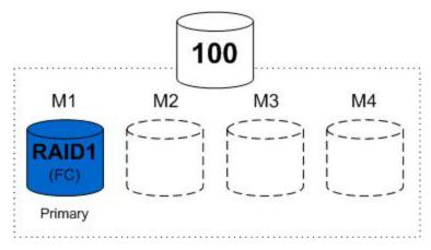
2. Move request is submitted and configuration lock is placed to do this. After this, the target RAID group is created in target Symmetrix tier and attached as secondary mirror M2 of the device.
