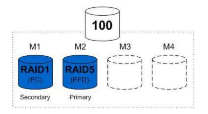
When the swap is done between mirror roles, the original RAID group is detached form the device and deleted. Also, the space previously used by RAID
