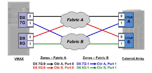
In the above example, the VMAX array is running DX emulation on odd director 7G and even director 8G which is within engine 4, i.e. the initial engine shipped when VMAX is ordered to EMC.
