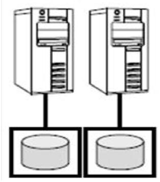
Figure 1: Direct Attached Storage [Server has its own internal/external storage]
