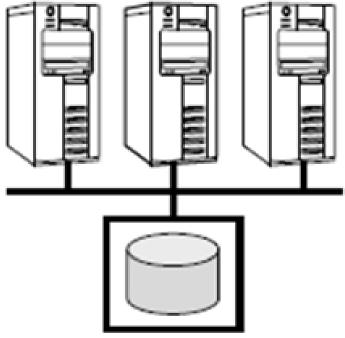
Figure 2: Network Attached Storage [Server connected over a network to the storage (file based)]
